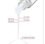
Identify the 4 depth marks on the needle (18 mm, 19 mm, 20 mm and 22 mm) to respect your working length.
